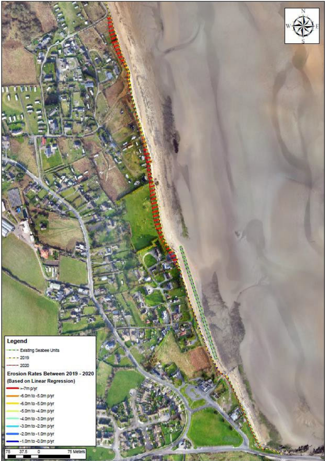
Figure 2.3: Erosion along the Burrow between 2019 and 2020
