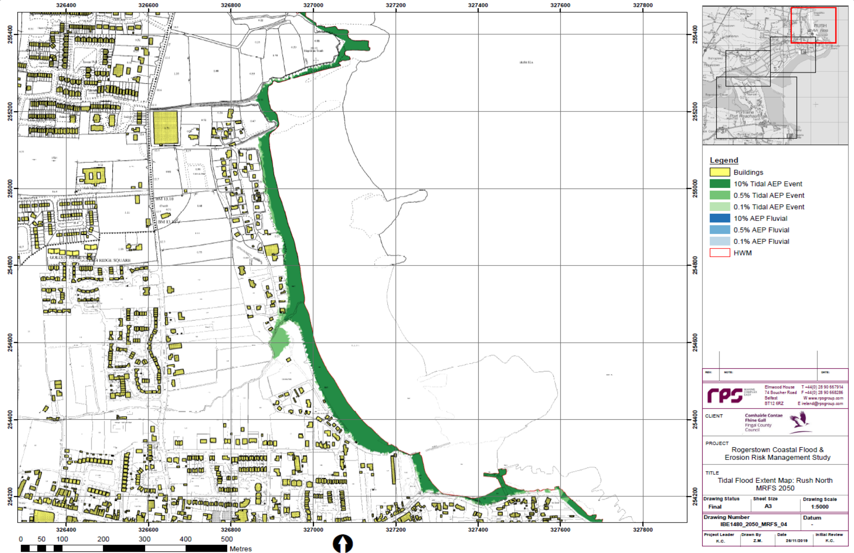
Figure 7.23: Tidal Flood Extent Map: Rush North - 2050 Medium Range Future Scenario (i.e. +0.20m sea level rise and c.2m of coastal retreat)
