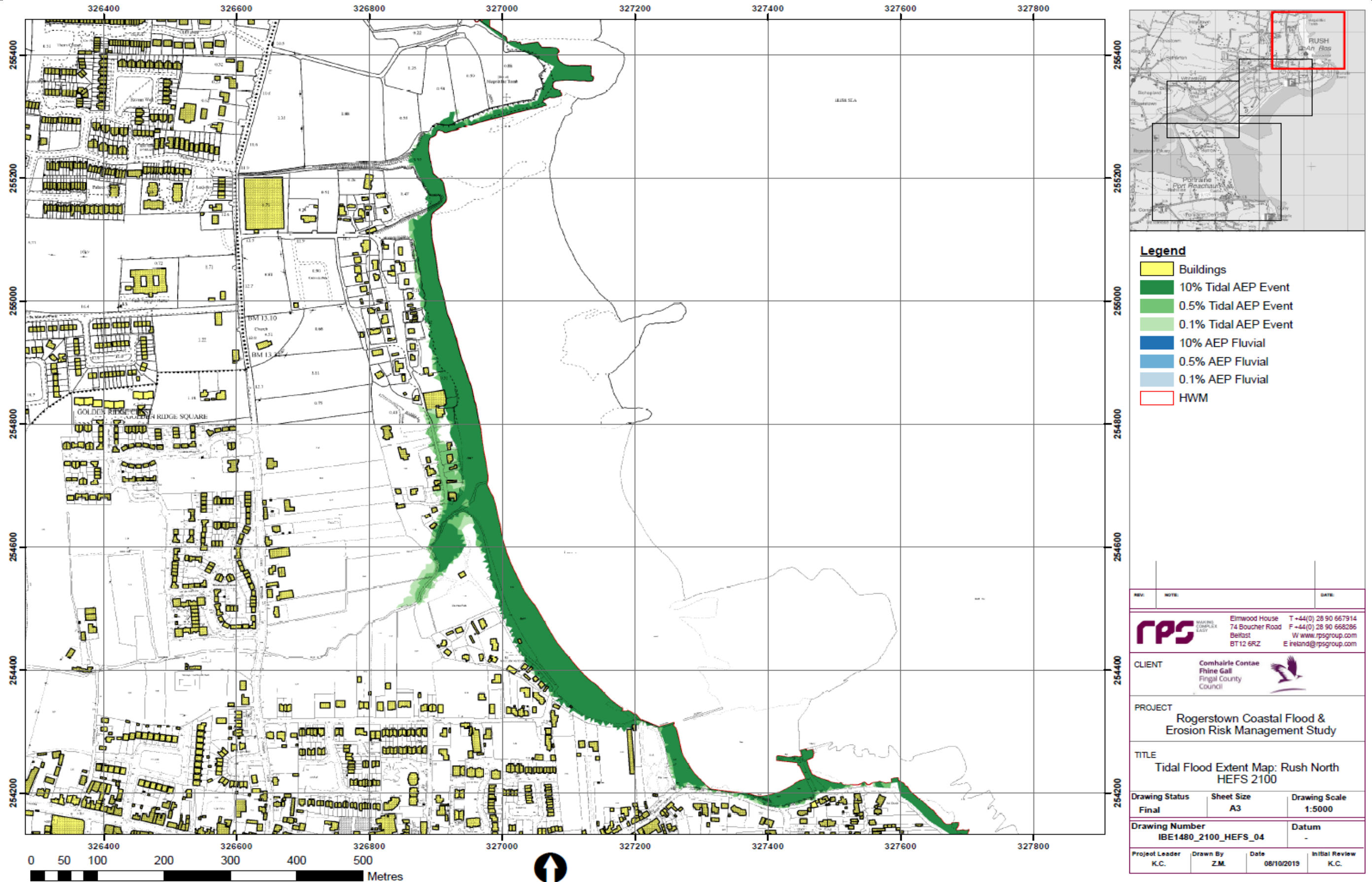
Figure 7.35: Tidal Flood Extent Map: Rush North - 2100 High End Future Scenario (i.e. +1.0m sea level rise and c.9m of coastal retreat)
