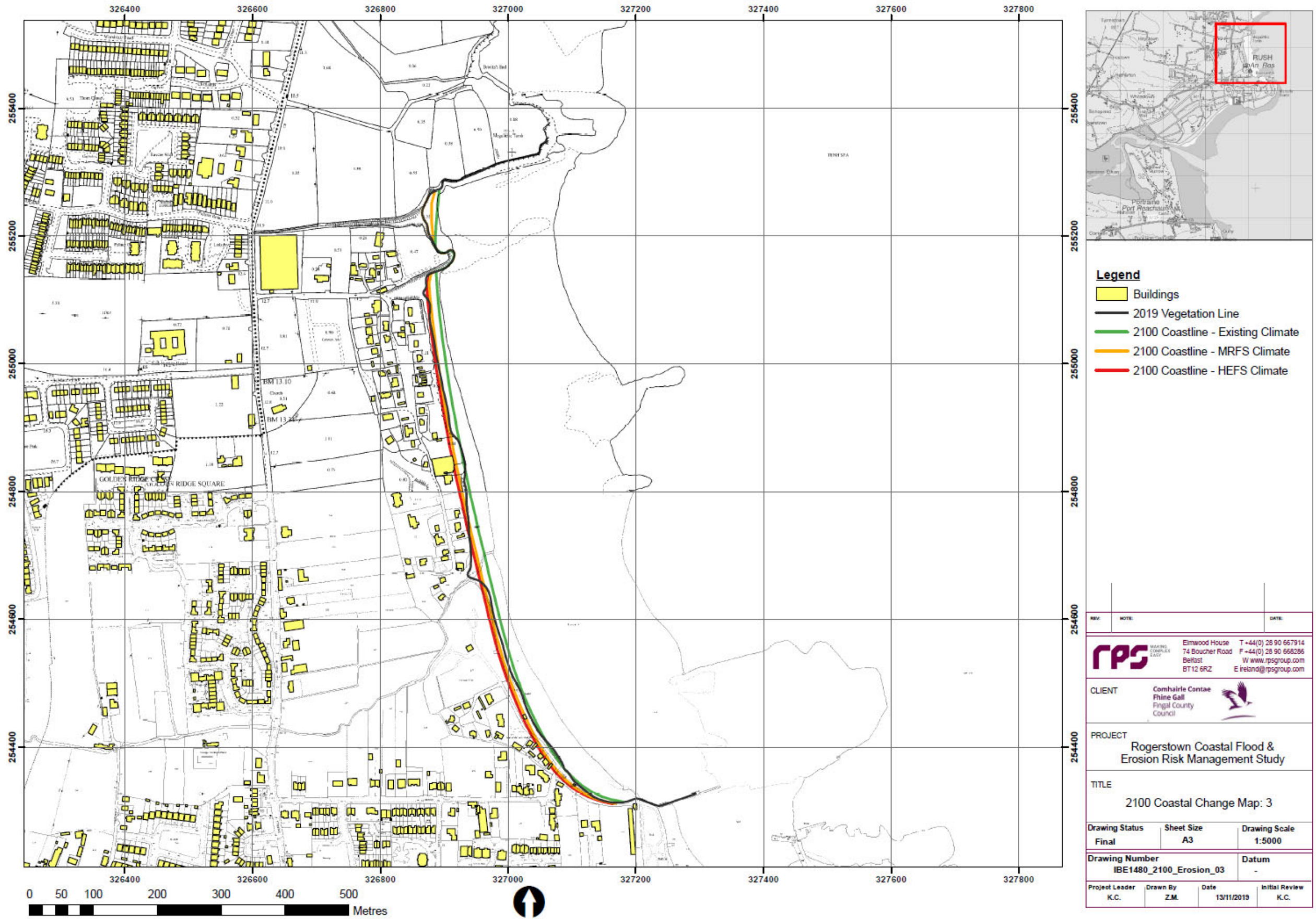
Figure 6.19: Projected coastal change at Rush North by 2100 based on various climate scenarios
