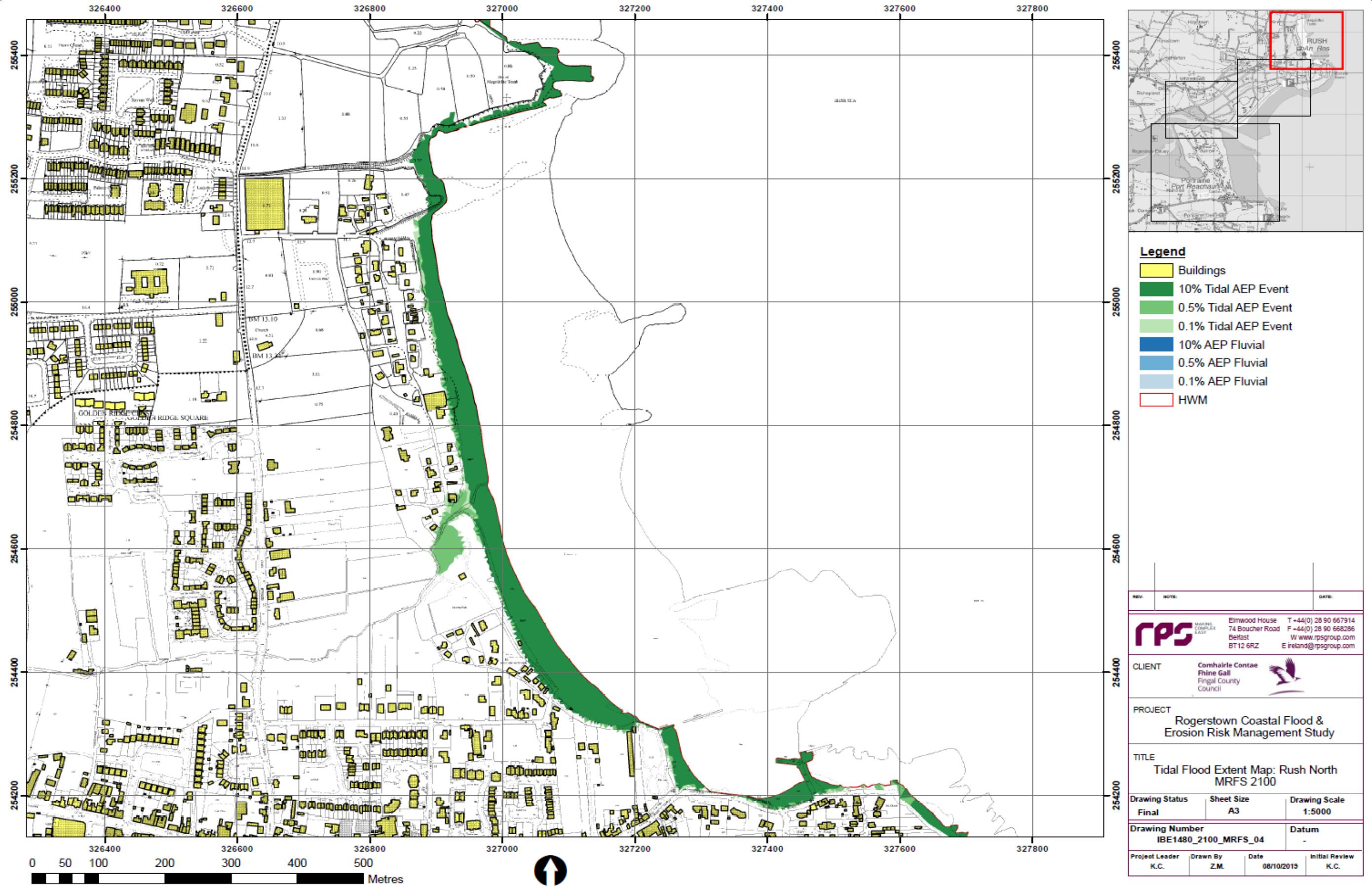
Figure 7.31: Tidal Flood Extent Map: Rush North - 2100 Medium Range Future Scenario (i.e. +0.50m sea level rise and c.4m of coastal retreat)
