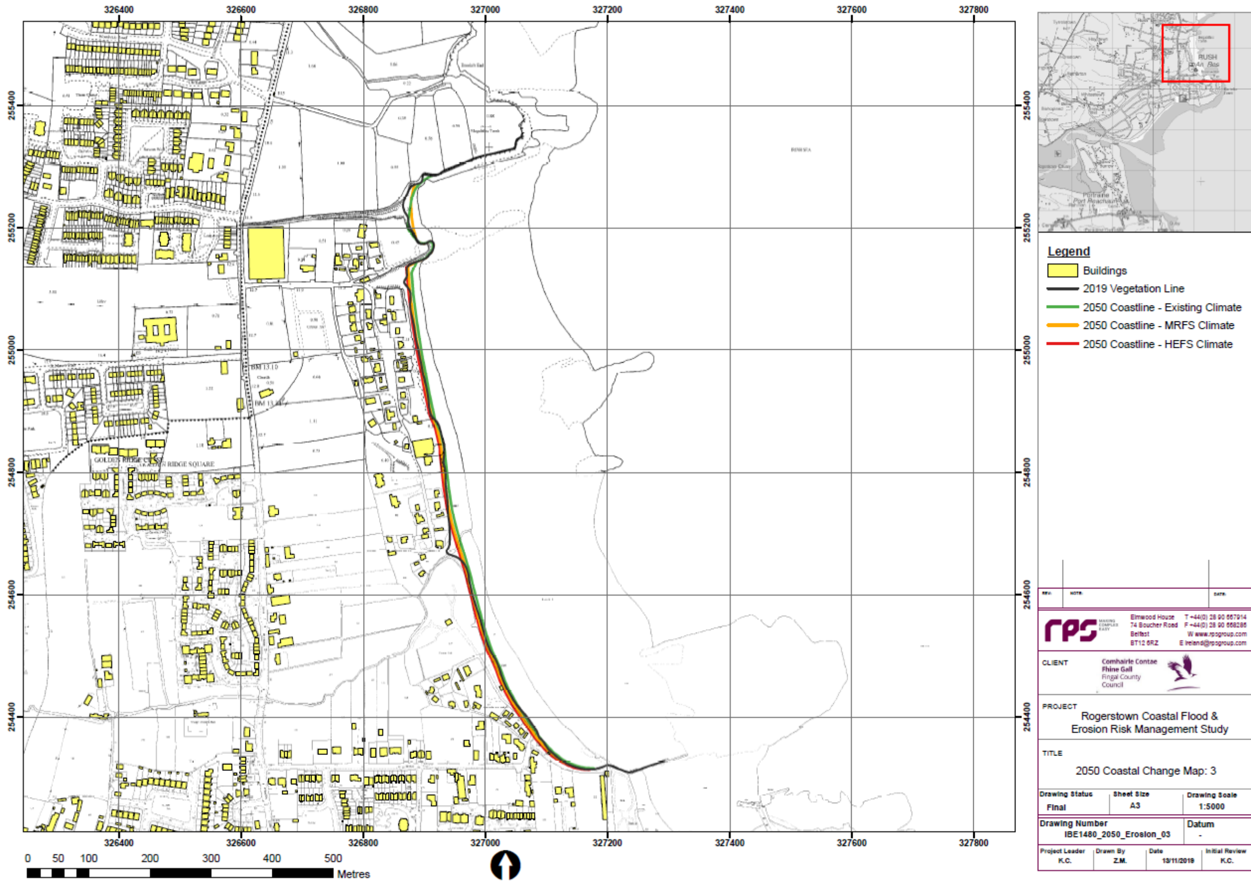
Figure 6.16: Projected coastal change at Rush north by 2050 based on various climate scenarios
