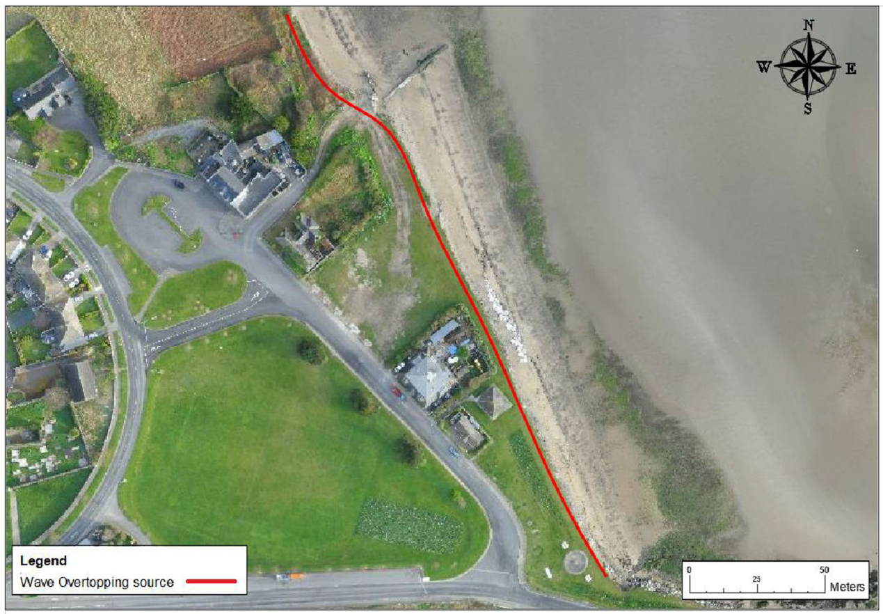
Figure 7.9: The corresponding discharge curve for each flood scenario was applied as a source term along the boundary illustrated in Figure 7.9.
